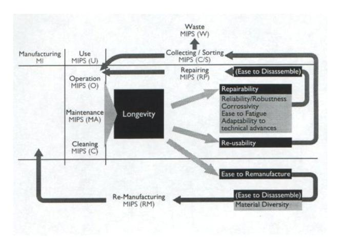
Fig 4: Survey of the different phases during the life of a product. The various types of possible MI and MIPS-(Material Input Per unit Service)-computations are indicated.
